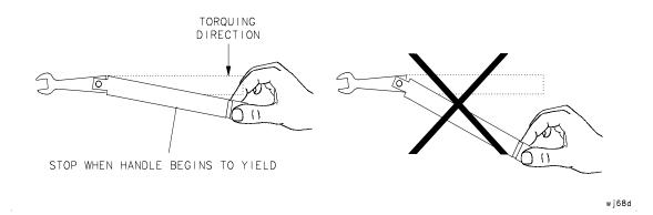
4. Apply force downward to the wrench handle. This applies torque to the connection *through* the wrench.
